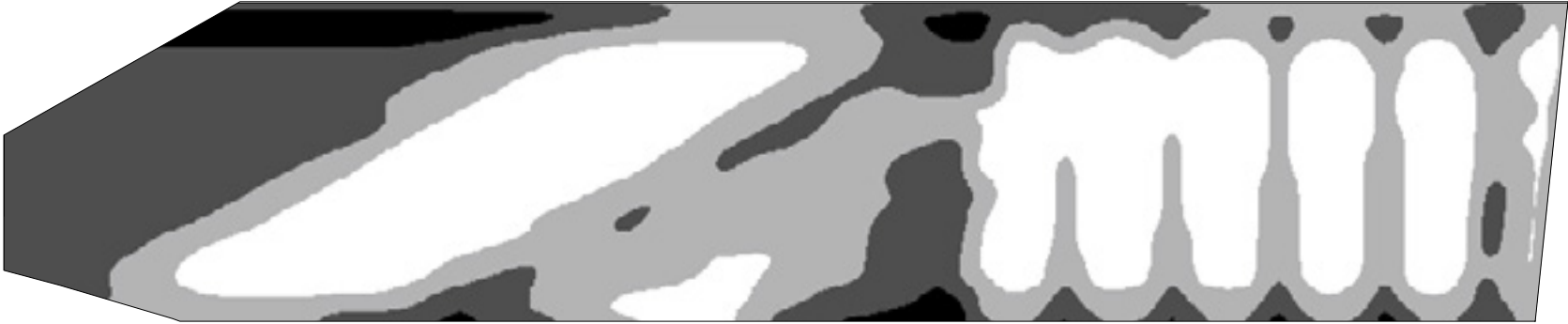
Depth map (distance between the surface of the topography and the sound mitigating layer)
