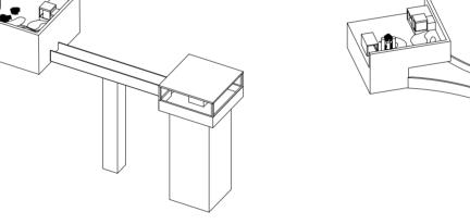
To create a more aesthetically pleasing building, the box and tower are turned 45 degrees and the bridge is given a hourglass-like shape. The corner of the box is also placed outside the roof of the existing building to create a separation of the prototype and
